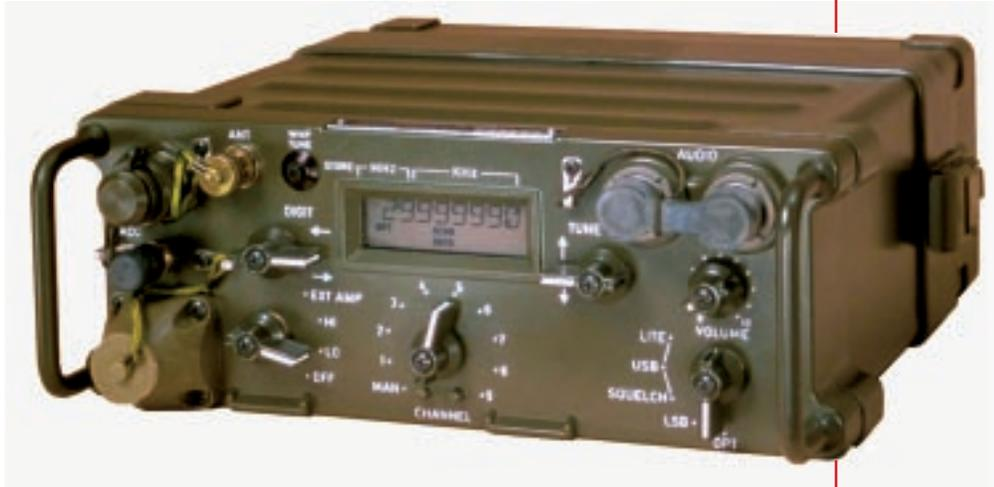
Datron's PRC1099A is an HF/SSB tactical manpack transceiver designed for demanding battlefield applications. It is a 20W radio operating over the full 1.6 - 30 MHz frequency range with 10 Hz resolution. The PRC1099A is rugged, lightweight, easy to use, and can be configured with numerous add-on ancillaries and accessories to create a wide variety of manpack, mobile, or base station systems.
