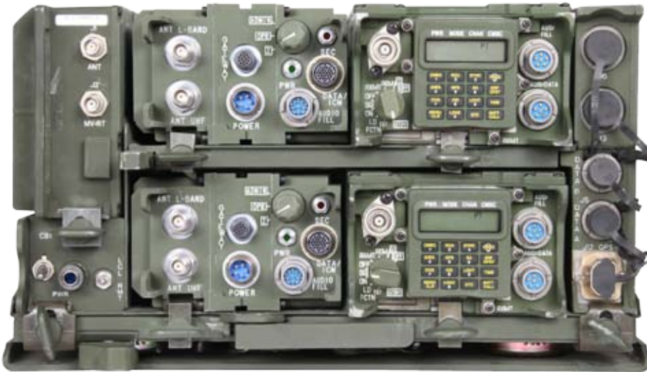
Four Channel Configuration: Dual SideHats and SINCGARS RT-1523s in VAA Mount
