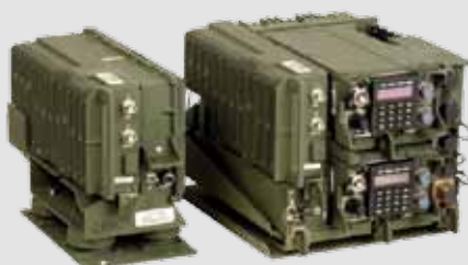
AN/VRC-92 Vehicular 50 W dual long-range (retransmit)- plus 2nd power amp and retrans cable
